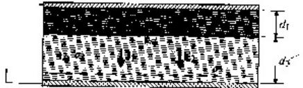
$$V = E_1 d_1 + E_2 d_2, \quad J = \sigma_1 E_1 = \sigma_2 E_2, \quad E_1 = \frac{\sigma_2 V}{\sigma_2 d_1 + \sigma_1 d_2}, \quad E_2 = \frac{\sigma_1 V}{\sigma_2 d_1 + \sigma_1 d_2}$$
