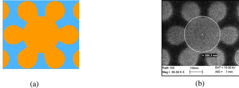
Fig. 8. Defect Fabrication error. (a) model for 496.5nm line with defect fabrication error. (b) SEM image of overlapped air pore and cavity for 496.5nm line
